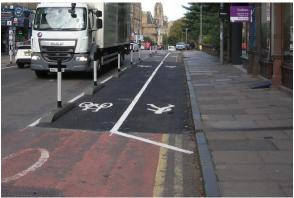
The pavement here is only 2.35m wide (ie less than the SDG 'absolute minimum' of 2.5m), with a Clear Walking Zone of just 1.3m. (ie less than the SDG 'absolute minimum' of 1.5m). There are long waits for the Green Man phase, during which large numbers of pedestrians can congregate in a way where it is impossible to maintain social distancing.
