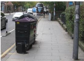
Although the pavement is reasonably wide here (3.2m), its utility is significantly constrained by the placement of communal bins, which reduce the Clear Walking Zone to just 1.2m (ie less than the SDG 'absolute minimum' of 1.5m).
