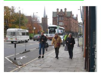
The pavement here is only 2.95m wide (ie less than the SDG 'general minimum' of 3m) and therefore the additional SfP space is welcome.
