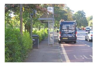
The pavement at the hedge here (foreground) is only 2m wide (ie the SDG 'absolute minimum'). At the litter bin the Clear Walking Zone is just 1.6m, while at the north end of the bus stop it is just 1.2m (ie significantly less than the SDG 'absolute minimum of 1.5m).
