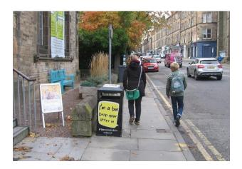
The pavement width here is only 1.85m (ie less than the SDG 'absolute minimum' of 2m), and the thoughtlessly-located litter bin reduces the Clear Walking Zone to just 1.25m (ie less than the SDG 'absolute minimum' of 1.5m) beside a very busy road.
