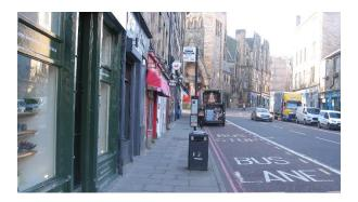
The pavement here is just 2.3m wide (ie less than the SDG 'absolute minimum' of 2.5m), and the Clear Walking Zone is even less, due to the litter bin.
