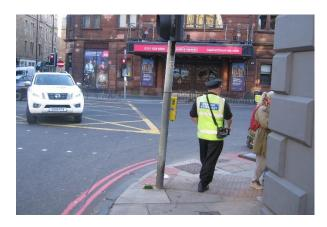
This is a very busy junction where the Leven Street pavement is only 2.4m wide (ie less than the SDG 'absolute minimum' of 2.5m) and the Gilmore Place pavement (pictured) is just 1.6m wide. There are long waits for the Green Man phase, during which large numbers of pedestrians can congregate in a way where it is impossible to maintain social distancing. This is a serious pinchpoint.
