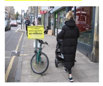
The pavement here is only 2.85m wide (ie less than the SDG 'general minimum' of 3m), and the Clear Walking Zone is reduced to just 2m by the signage pole / informally-parked bike (and the yellow SfP sign!).
