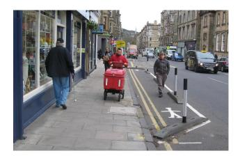
The pavement here is only 2.35m wide (ie less than the SDG 'absolute minimum' of 2.5m) and therefore the additional 1.3m SfP space is very welcome, not least as goods are sometimes on display on the pavement outside this shop. The extra width also narrows the width of (informal) crossing of the Morningside Road carriageway on a long section without formal crossing facilities.
