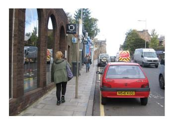
The pavement here is only 1.8m wide (ie substantially less than the SDG 'absolute minimum' of 2.5m) and the Clear Walking Zone is just 1.5m at the pole.
