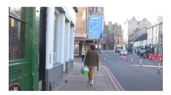
The pavement here is just 2.35m wide (ie less than the SDG 'absolute minimum' of 2.5m). While the current traffic management works associated with the ScotMid reconstruction site opposite preclude early action, this is a pavement which needs widening.
