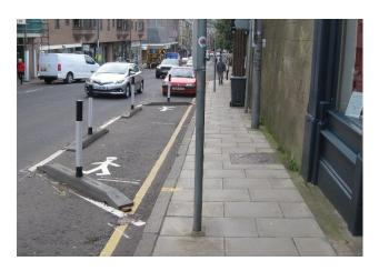
The pavement here is only 1.8m wide (ie substantially less than the SDG 'absolute minimum' of 2.5m) and the Clear Walking Zone is just 1.5m at the pole, therefore the additional SfP space is most welcome.
