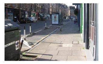
The pavement here is just 2.8m wide (ie less than the SDG 'general minimum' of 3m) and therefore the additional SfP space is welcome, close to the bus stop.
