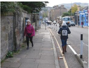
The pavement here is only 2.05m wide (ie significantly less than the SDG 'absolute minimum' of 2.5m) and the Clear Walking Zone is just 1.7m in places – therefore the additional 0.95m SfP space is most welcome.
