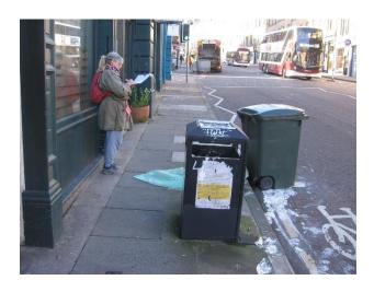
The pavement here is just 1.35m wide (ie substantially less than the SDG 'absolute minimum' of 2.5m), and the Clear Walking Zone is even less, due to the inappropriately located litter bin.
