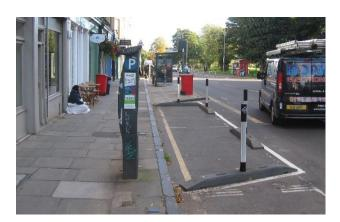
The pavement here is only 2.8m wide (ie less than the SDG 'general minimum' of 3m), and the Clear Walking Zone is just 1.85, due to the parking ticket machine, and therefore the additional SfP space is welcome.
