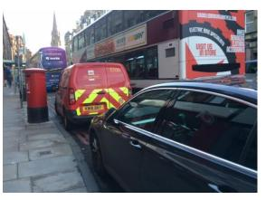
The SfP space here provides a useful 2m addition where the pavement proper is just 3m wide, ie significantly less than the Street Design Guidance (SDG) 'desirable minimum' of 4m or wider. The extra space is useful not just for 'movement' but also for pedestrians to stop and chat in 'social' space without obstructing others. This location is very busy with school students in the morning peak, at lunchtimes and mid-afternoon.
