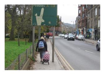
The pavement here is only 1.8m wide (ie substantially less than the SDG 'absolute minimum' of 2.5m) and the Clear Walking Zone at the poles is just 1.05m (ie substantially less than the SDG 'absolute minimum' of 1.5m).
