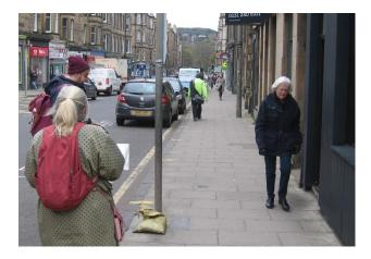
The pavement here is only 2.2m wide (ie significantly less than the SDG 'absolute minimum' of 2.5m) and the Clear Walking Zone is just 1.7m at the pole.
