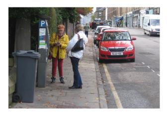
The pavement width here is only 1.9m (ie less than the SDG 'absolute minimum' of 2m), and the parking ticket machine reduces the Clear Walking Zone to just 1.5m.
