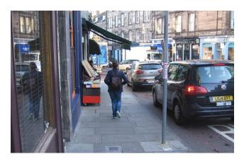
The pavement here is just 2.3m wide (ie less than the SDG 'absolute minimum' of 2.5m), and the Clear Walking Zone is even less, due to the goods on display outside the fruit shop. Section 129(9) of the Road Scotland Act 1984 forbids the placement of goods for sale on the public sections of the street. If alerted to such a problem, the Council can issue a statutory notice to the offending business and action then taken if they fail to comply.
