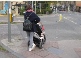
The pavement width beside Costa (left photo) at the waiting area for the crossing is only 2.2m, and the Clear Walking Zone is just 1.5m. The width of the pedestrian island part-way across Colinton Road (right photo) ranges from 1.7m to 3.2m.
