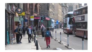
A useful 2.1m addition where the pavement proper is just 2.65m wide, ie significantly less than the SDG 'desirable minimum' of 4m or wider.
