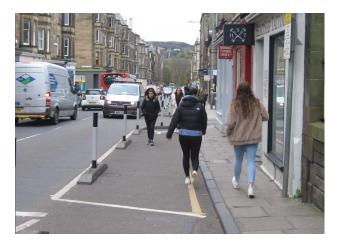
This is one of the most valuable improvements made by the SfP project along the A702 corridor. The pavement proper is only 1.25m wide (ie half the SDG 2.5m 'absolute minimum') and therefore the additional 1.75m SfP space is very welcome, taking the entire pedestrian space width up to the 3m SDG 'general minimum', albeit split in two levels.
