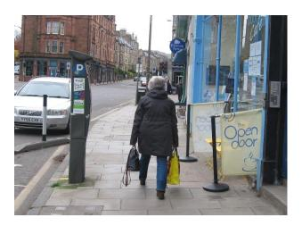
The pavement here is only 2.85m wide, and the tables & chairs and parking ticket machine reduce the Clear Walking Zone to just 1.6m.
