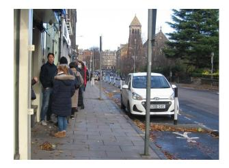
The pavement here is only 2.65m wide (ie less than the SDG 'general minimum' of 3m), and this is a location where queuing on the pavement is common.
