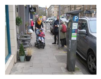
The pavement here is only 2.4m wide (ie less than the SDG 'absolute minimum' of 2.5m) and the parking ticket machine, tables & chairs and poles reduce the Clear Walking Zone in places to 1.45m.
