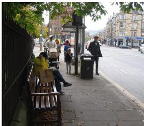
The pavement at the bus stop is only 2.9m wide, with a Clear Walking Zone of just 1.7m. At the bench the pavement is only 2.4m wide, with a Clear Walking Zone of just 2m.
