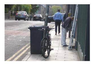
The pavement here is only 1.9m wide (ie substantially less than the SDG 'absolute minimum' of 2.5m), with a Clear Walking Zone of just 1.2m. (ie substantially less than the SDG 'absolute minimum' of 1.5m). There are long waits for the Green Man phase, during which large numbers of pedestrians can congregate in a way where it is impossible to maintain social distancing.
