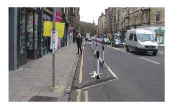
The pavement here is only 2.7m wide, and the signage pole (and SfP sign), and therefore the additional 1.4m SfP space is welcome.
