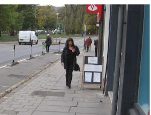
The pavement here is only 2.8m wide (ie less than the SDG 'general minimum' of 3m) and therefore the additional SfP space is welcome. However, an illegally-sited advertising board partly obstructs the pavement proper.
