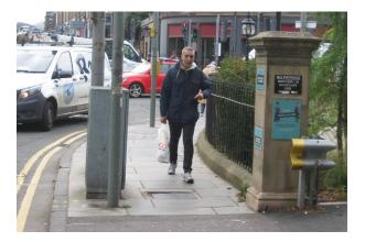
The pavement here is only 2.3m wide (ie less than the SDG 'general minimum' of 2.5m), despite this being one of the busiest pedestrian junctions on the entire corridor) and the poles / grey utility box reduce the Clear Walking Zone to just 1.4m (compared to the SDG 'absolute minimum' of 1.5m).
