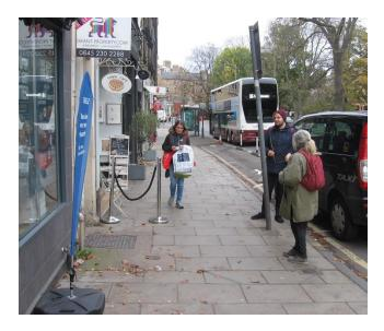
The pavement here is 3.15m wide, but the Clear Walking Zone at the signage pole is just 1.4m wide (ie less than the SDG 'absolute minimum' of 1.5m).
