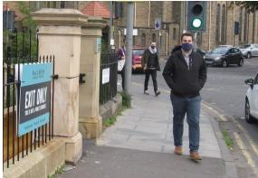
The pavement width at the queuing area for this important pedestrian crossing is only 2.3m (ie less than the SDG 'general minimum' of 2.5m), and the Clear Walking Zone between the two poles (left photo) is just 1.4m, compared to the SDG 'absolute minimum' of 1.5m.
