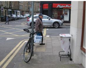
The pavement here is only 1.9m wide (ie substantially less than the SDG 'absolute minimum' of 2.5m) and, due to informal cycle parking and the shoe recycling bin, the Clear Walking Zone is just 0.65m (ie less than half the SDG 'absolute minimum').
