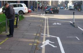
The pavement here is just 2.1m wide (ie significantly less than the SDG 'absolute minimum' of 2.5m), with a Clear Walking Zone of just 1.6m at the litter bin. The additional 1m walking lane is therefore very welcome, but this still leaves the total width for pedestrians at substantially less than the SDG 'desirable minimum' of 4m or wider, and the width is at two levels rather than being continuous.
