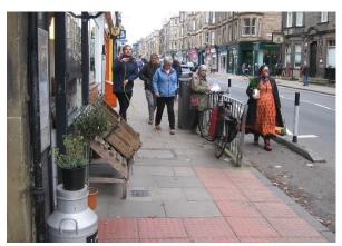
The pavement proper here is only 2.6m wide, and due to various items of pavement clutter (and goods on display) the Clear Walking Zone is reduced to 1.5m in places – and therefore the additional 1.1m SfP space is welcome. The latter also reduces the width of carriageway to cross at the pedestrian crossing. However the total width available for pedestrians is split both horizontally (by
