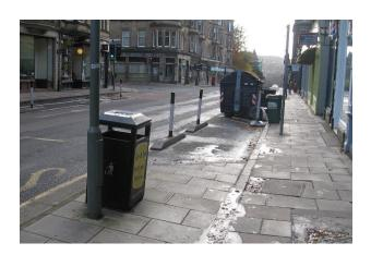
The pavement here is only 1.9m wide (ie substantially less than the SDG 'absolute minimum' of 2.5m) and therefore the additional 1.8m SfP space is very welcome as a 'social' space and also a 'movement' space contiguous with the bus stop 'build-out'.
