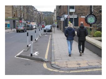
The pavement here is only 2.25m wide (ie significantly less than the SDG 'absolute minimum' of 2.5m) and therefore the additional 1.05m SfP space is welcome.
