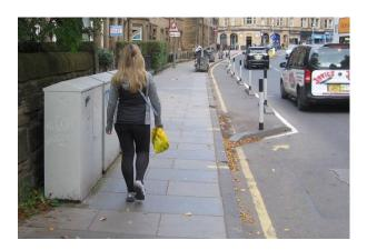
The pavement narrows to only 2.15m here (ie less than the SDG 'absolute minimum' of 2.5m), and the grey utility boxes reduce the Clear Walking Zone to just 1.6m.
