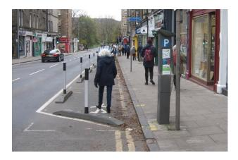
The pavement here is only 2.7m wide (ie only just wider than the SDG 'absolute minimum' of 2.5m) and therefore the additional 2m SfP space is welcome.
