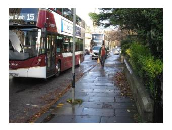
The pavement here is only 2.2m wide (ie less than the SDG 'absolute minimum' of 2.5m, which is 'only allowed in short sections).
