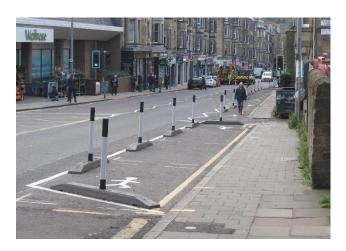
This is one of the most valuable improvements made by the SfP project along the A702 corridor. The pavement proper is only 2.15m wide (ie significantly less than the SDG 2.5m 'absolute minimum') and therefore the additional space is very welcome for pedestrians.
