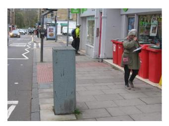
The pavement here is 3.15m wide, but the utility cabinet reduces the Clear Walking Zone to 2.25m.
