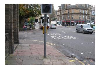
The pavement here is only 2.8m wide (ie less than the SDG 'general minimum' of 3m), and the Clear Walking Zone is just 1.8m.
