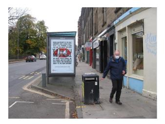
The bus build-out helps to relieve a pavement which is otherwise only 2.7m wide, but the inappropriately located litter bin reduces the Clear Walking Zone to just 1.8m
