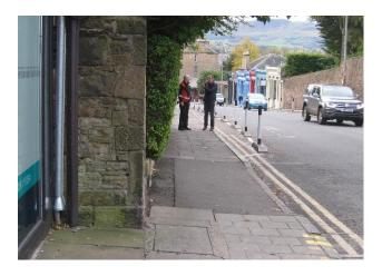
Immediately south of the southbound bus stop at Church Hill, the pavement narrows to just 2.05m, but vehicle access to a property on the left prevented the SfP space measure (see Location 35E2) being extended uphill to reach the wider pavement.
