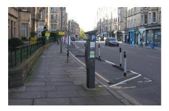
The pavement here is only 2.7m wide (ie only just wider than the SDG 'absolute minimum' of 2.5m) and the Clear Walking Zone is just 1.85m is places – therefore the additional SfP space is welcome as a 'social' space. Its utility as a 'movement' space is less clear, as it is a short length, discontinuous with the next short SfP space a short distance to the south (see 16E below).
