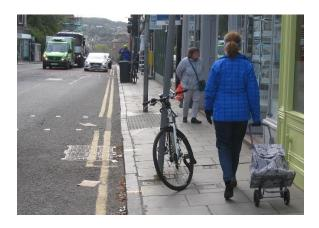
The pavement here is only 1.85m wide (ie substantially less than the SDG 'absolute minimum' of 2.5m), with a Clear Walking Zone of just 1.5m. There are long waits for the Green Man phase, during which large numbers of pedestrians can congregate in a way where it is impossible to maintain social distancing.
