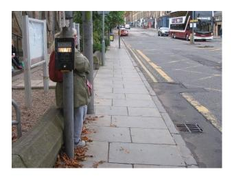
The pavement width here is only 1.8m (ie less than the SDG 'absolute minimum' of 2m). Pedestrians can feel very vulnerable at this location on such a narrow pavement strip, with southbound vehicles on Morningside Road passing at speed less than a metre away. There are long waits for the Green Man phase, during which large numbers of pedestrians can congregate in a way where it is impossible to maintain social distancing.
