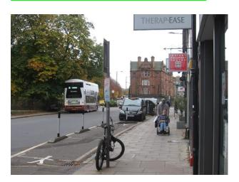
The pavement here is only 2.9m wide and the Clear Walking Zone is reduced by the informal bike parking and pole – and therefore the additional 2m SfP space is welcome.
