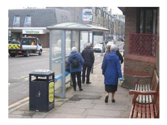
This is one of the most significant pedestrian pinchpoints on the A702 corridor. The pavement is only 2.5 wide (ie the SDG 'absolute minimum') and the Clear Walking Zone at the bus stop is just 1.65m – making it impossible to socially distance for much of the time.
