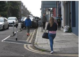
The pavement here is only 2.1m wide (ie less than the SDG 'general minimum' of 2.5m). This is often a busy section of pavement and queuing outside the Post Office is common, therefore the additional SfP space is welcome as a 'social' space and also a 'movement' space.
