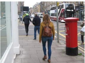
The junction of Morningside Park and Morningside Road has been an accident black-spot and the pavements here are narrow: only 1.8m beside the tactile paving for crossing Morningside Park (left photo) and 2.8m on the main pedestrian route (up Morningside Road, right photo), with a Clear Walking Zone of just 1.8m to the post box.
