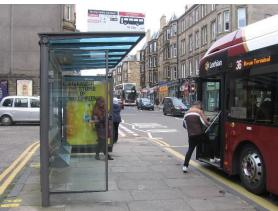
This location is poorly designed for pedestrians, both those walking up or down Morningside Road and those boarding or alighting from buses (this is normally a busy bus stop). The advertising screen at the north end of the JC Decaux shelter reduces the Clear Walking Zone to just 1.7m at this pinchpoint.
