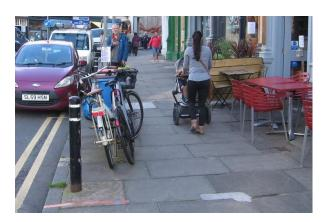
Although the pavement is reasonably wide here, its utility is significantly constrained by a combination of formal cycle parking and tables & chairs, leaving a Clear Walking Zone of just 1.4m on a pavement section regularly busy with pedestrians.
