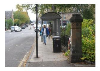
The pavement width here is only 2.15m (ie less than the SDG 'absolute minimum' of 2.5m) at a location where queuing (for buses) is frequent, and the Clear Walking Zone is just 1.35-1.45m (ie less than the SDG 'absolute minimum' of 1.5m).
