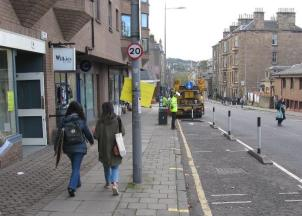
While the pavement here is reasonably wide, much of it is on a slope rising up to the shop entrances (right photo) which is unsuitable for more infirm pedestrians to walk along. On the horizontal pavement, the Clear Walking Zone is as narrow as 1.25m and 1.85m in places, and therefore the additional SfP space is welcome.
