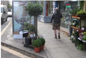
The pavement proper here is only 2.6m wide, and due to the depth of goods on display here, the Clear Walking Zone is only 1.2m in places (ie significantly less than the SDG 'absolute minimum' of 1.5m). Therefore the additional SfP space is welcome, albeit that the total width available for pedestrians is split into two levels rather than being continuous.
